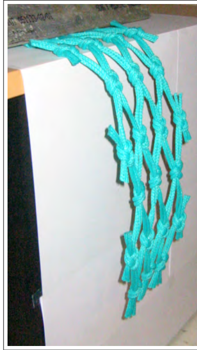
Figure 3.14: The net bends under its own weight, which highlights the bending stiffness of the net.
