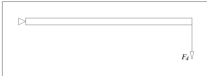
Figure 2.7: This bar is articulated around its left extremity. A vertical force ( F_4 ) is applied on the right extremity. This unstretched bar displays a zero stiffness along the vertical.
